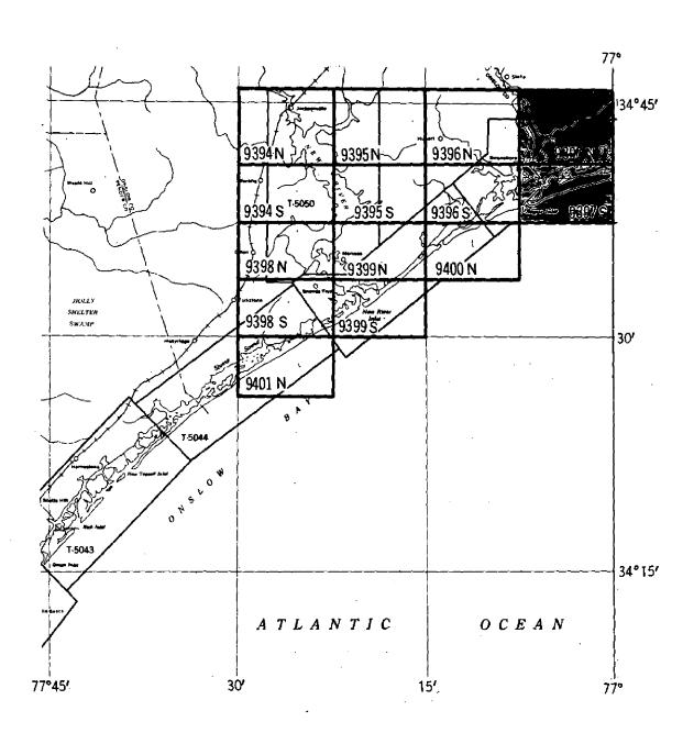
Project Ph-58(49), a topographic mapping survey, consists of 8 quadrangles numbered T-9394 to T-9401, inclusive. The area of the project is located in the vicinity of the town of Swansboro and New River, N.C., and extends from the coastline between longitudes 77° 00' and 77° 30' northward to latitude 34° 46'. To the east it junctions with Ph-5(45) - a topographic and shoreline mapping project.
